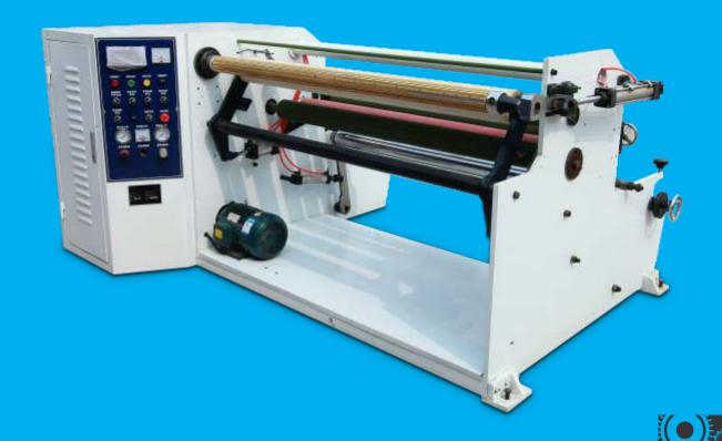
This machine can change any diameter of rewinder shafts; One-click filling deflated; intelligent control plate; Magnetic powder type winding control; rewinding smoothly; easy to control.
