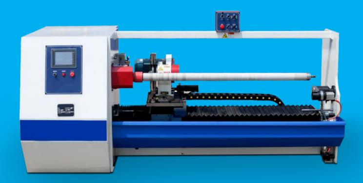
The machine uses the round blade, it can cooling and lubrication by itself. pneumatic controls feed-in cutting blade, step motor controls the cutting width, manually adjust the angle of cutting.
