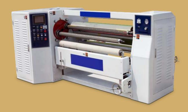
This machine can change any diameter of rewinder shafts; One-click filling deflated; double shafts exchange winding, high speed and high efficiency; intelligent control plate; Magnetic powder type winding control; rewinding smoothly. LED touch screen data input and display, easy to control. Unwinding parts can choose to add the silencer device; and also choose to add the Hydraulic automatic feeding device. (According to cilent's requirement)
